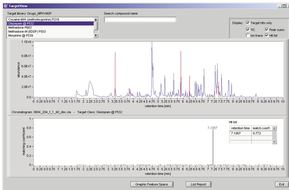
**Figure 3:** Software interface for analysis of the urine sample. The upper window shows the baseline-compensated TIC, with target drugs marked by the red bars. The lower window shows the target match for diazepam, with a match coefficient of 0.772.
