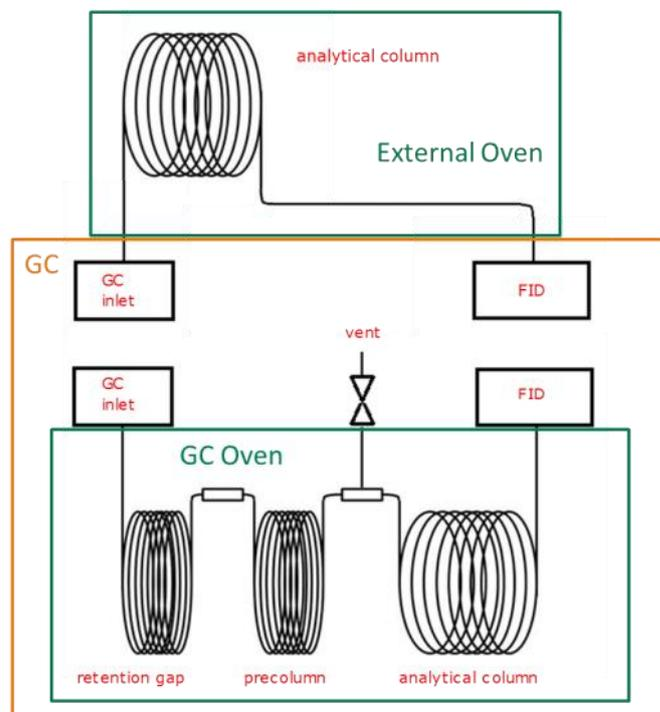
Figure Three: Column Configuration ASTM D7756 & D2163
