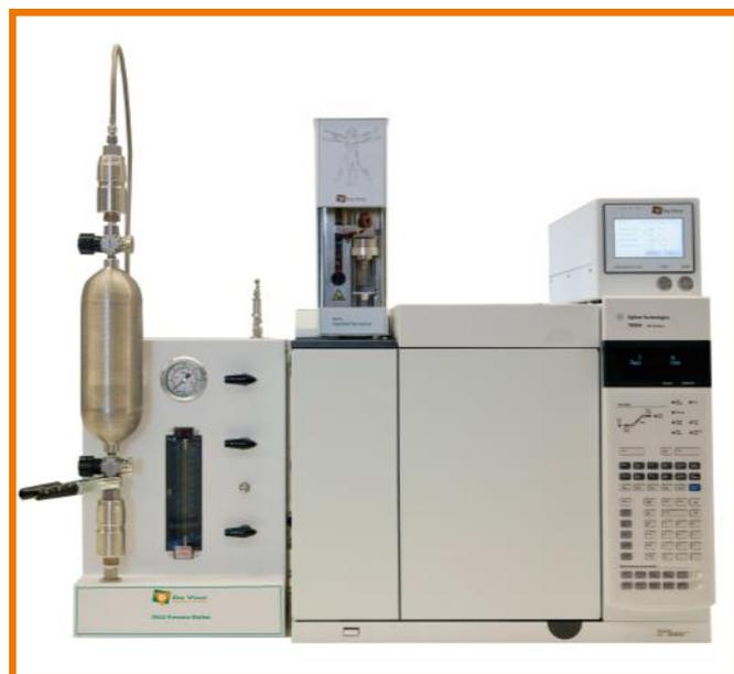
Figure One: Agilent GC & DVLS Liquefied Gas Injector
