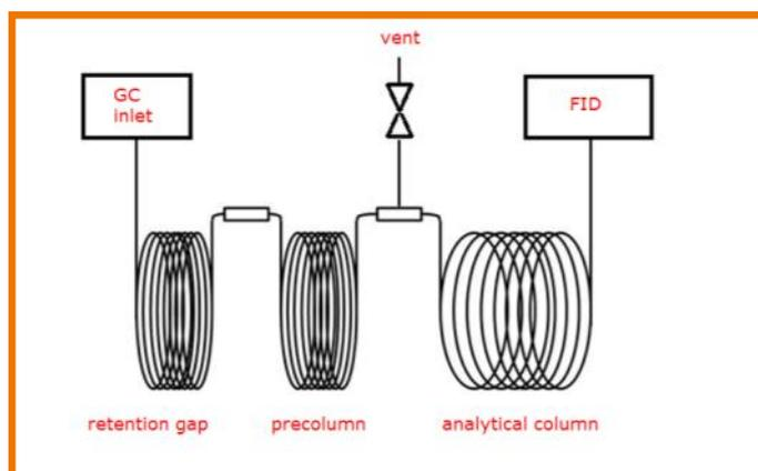
Figure Two: Column Configuration ASTM D7756
