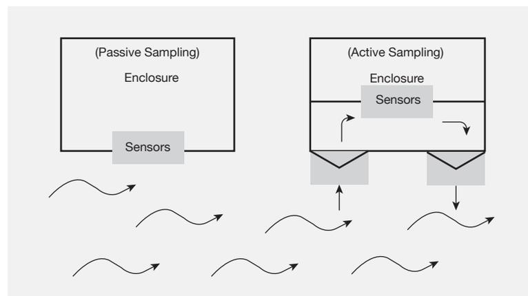
Sensor-based air quality monitoring systems have also evolved with technological advancements. Conventional sensor-based systems had their sensors exposed to ambient atmospheric conditions known as passive sampling-based sensors. Due to which, ambient environmental conditions such as heavy dust, high wind speed, temperature, and humidity affects directly exposed sensors. Such systems are highly affected by the above mentioned environmental con-
